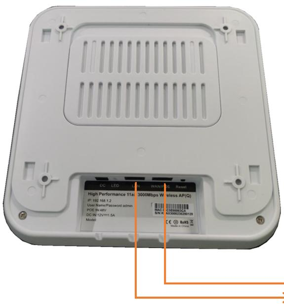
1. **POE Power Supply Port:** The adapter powers the gateway through the Ethernet cable.
