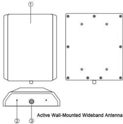
① Active Antenna Amplifier Module: Amplifies the received signal. ② RF Indicator Light: Shows the antenna operating status. ③ BNC Connector: Connects the antenna using a coaxial cable.
